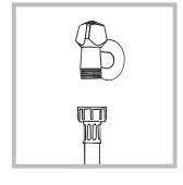
2. Connect the inlet hose by screwing it to a cold water tap using a 3/4 gas threaded connection (see figure).
